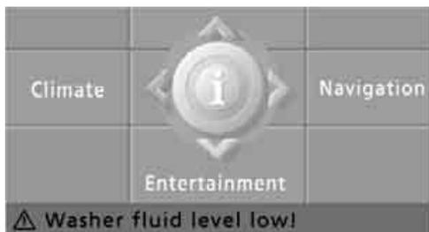
Text messages at the bottom edge of the Control Display explain the meaning of the displayed indicator and warning lamps.
