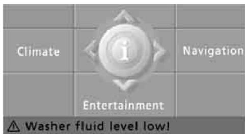
Text message at the bottom edge of the Control Display explain the meaning of the displayed indicator and warning lamps.
