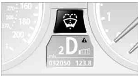
▲ This symbol means that a Check Control message has been generated. The symbol continues to be visible even when the Check Control message disappears after a short time. The warning lamps and text messages are stored and can be displayed later, also refer to page 76.
