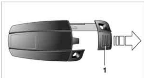
Press button 1 to unlock the key.
