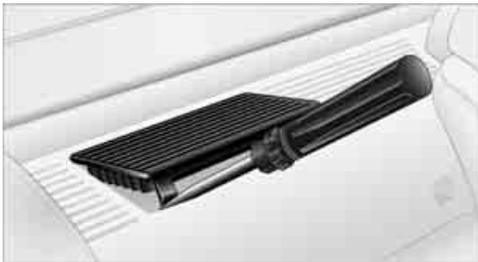
2. Insert the Allen wrench as far as possible into the opening and turn firmly in the direc-
