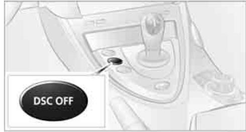
Press the DSC OFF button; the DSC indicator lamp lights up continuously. DSC and MDM are deactivated.
