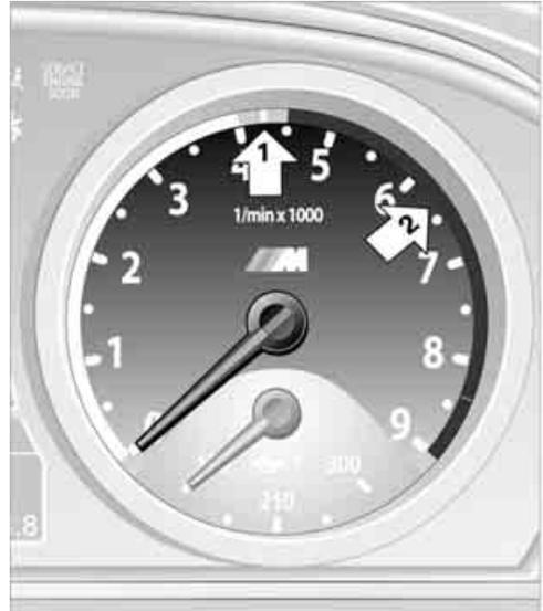
The advance warning field, arrow 1, and the red warning field, arrow 2, change depending on the engine temperature. As the engine temperature rises, the permissible engine speed also increases. Avoid allowing the engine speed to rise as far as the orange warning field whenever possible.
