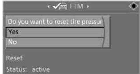
The message "resetting FTM ..." is displayed for a few seconds. The warning lamp in the instrument cluster lights up yellow for a few seconds.
