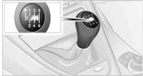
**!** While shifting in the 5th/6th gear lane, press the gearshift lever toward the right, otherwise accidental shifting into the 3rd or 4th gear could result in engine damage. ◀
