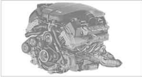
With a 305 cu in/5 liter displacement, the high-speed V10 engine generates a maximum output of 373 kW and a maximum torque of 384 lb ft/520 Nm. Its spontaneous response characteristics yield a very broad usable engine speed range. At the maximum engine speed of 8,250 rpm, the flow of fuel is interrupted in order to protect the engine. Due to the powerful engine dynamics, when the vehicle is at rest, the maximum engine speed is limited to 7,000 rpm.
