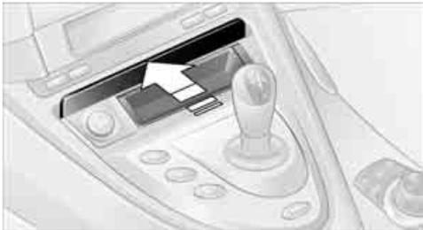
Press the opened cover beyond the resistance point, refer to arrow: the ashtray lifts up for removal.
