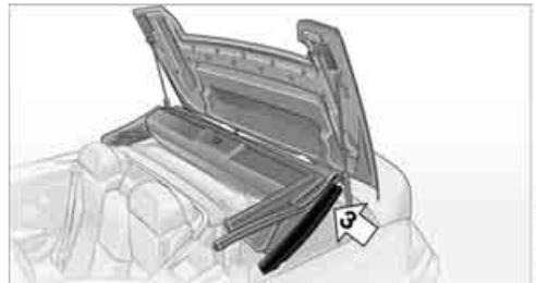
3. Together with the other person, pull the two sides of the convertible top out simulta-
