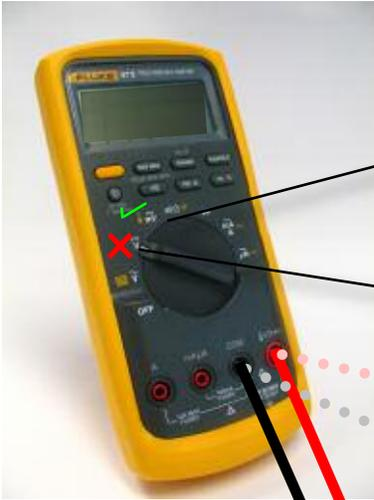
Using the Volts [V] setting will not render the needed accuracy for this measurement! Instead, use the millivolt [mV] setting.
