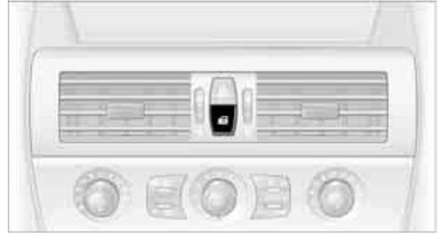
This button serves to unlock or lock doors and the luggage compartment lid, but does not activate the anti-theft system. The fuel filler door remains unlocked.
