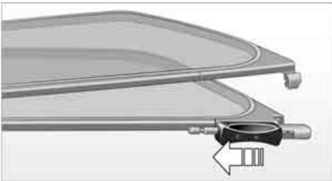
1. Push the handle of the securing pin on the wind deflector on the left side of the vehicle all the way back and release the locking mechanism.
