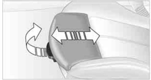
Pull the lever and adjust the thigh support in the longitudinal direction.
