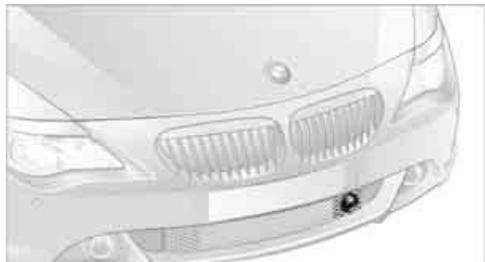
The function of the camera may be affected by heavy rain and fog, dirt, snow or ice on the lens. When this occurs, the displayed image on the Control Display may become gray.
