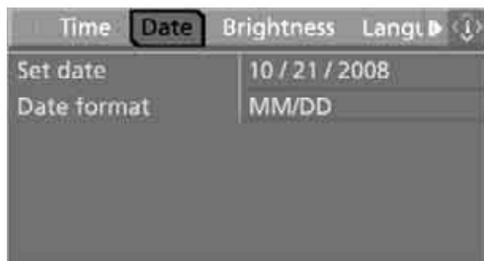
2. Select "Set date" and press the controller. The first section of the date display is highlighted, in this case the month
