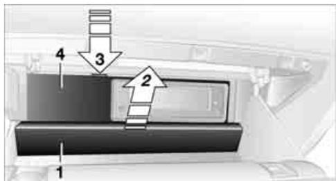
2. Press the coupling downward, arrow 3, and fold the lid 4 forward.
