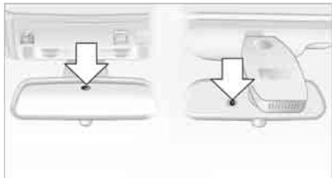
The interior mirror is provided with two photocells to control its automatic dimming function. One is integrated into the mirror glass, refer to arrow, while the other is located at a position slightly offset from this on the back of the mirror housing.
