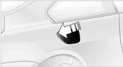
To open and close: briefly press the rear edge of the fuel filler door.
