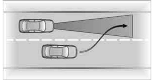
When a vehicle moves from an adjacent lane into your lane, active cruise control will not recognize this vehicle until it is fully in your lane ahead of your vehicle.
