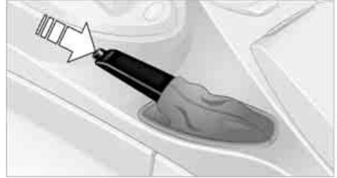
Pull slightly upwards, press the button and lower the lever.
