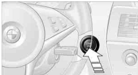
Briefly pressing the Start/Stop button several times switches the radio readiness or the ignition on and off.
