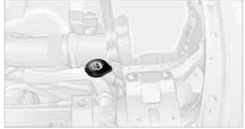
All washer jets are supplied from one reservoir. Fill with water and – if required – with a washer antifreeze, according to manufacturer's recommendations.
