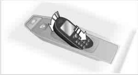
The mobile phone's battery is charged with the ignition lock at radio readiness or higher or with the steering unlocked.
