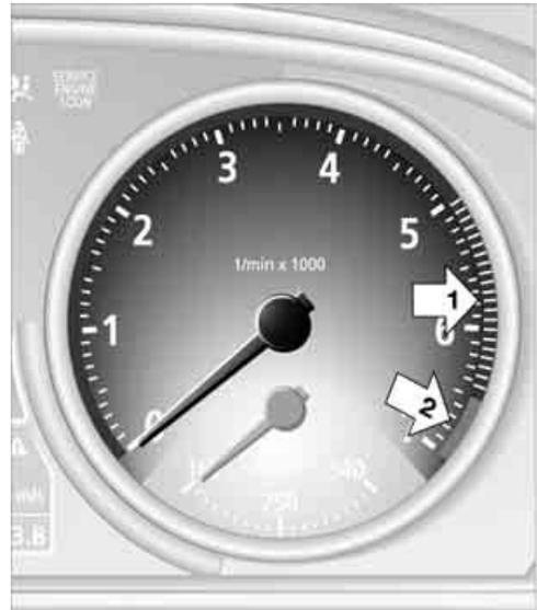
The white-striped advance warning field, arrow 1, changes depending on the engine temperature. The segments disappear in sequence as the engine warms to its normal operating temperature.
