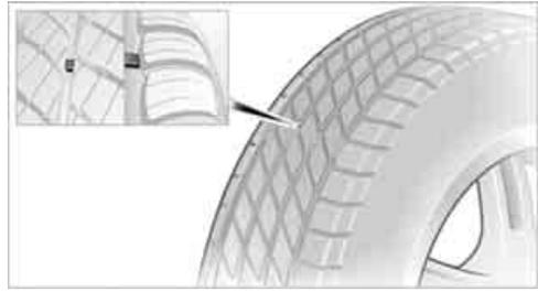
Wear indicators at the tread-groove base, refer to arrow, are distributed over the tire's circumference and are marked on the side of the tire with TWI – Tread Wear Indicator. If the tire tread has been driven down to the wear indicators, a tread depth of 0.063 in/1.6 mm has been reached.
