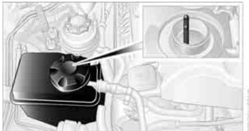
1. The engine must be at ambient temperature.
