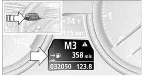
To display the information, press the BC button in the turn signal lever from radio readiness.
