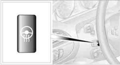
Press the button with the ignition switched on. The indicator lamp in the button lights up when the steering wheel heater is switched on.
