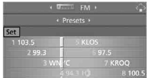
With some stations the digital signals are not transmitted simultaneously with the analog signals. If you are in an area in which the selected station is not continuously received digitally, playback switches between analog and digital reception. This can result in repetitions or interruptions. In this case it may be advisable to deactivate digital radio reception.
