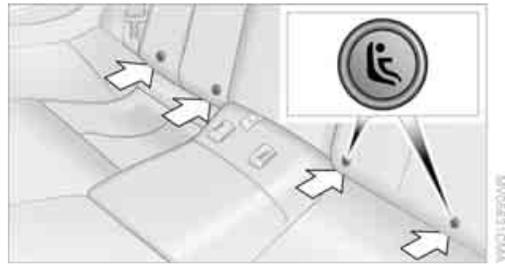
The mountings for the LATCH child-restraint fixing system are located under the points marked with the symbols. They are not visible from the outside.
