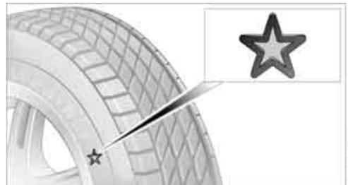
BMW recommends particular tire brands for each tire size. You can recognize these from the clearly visible BMW marking on the tire sidewall.
