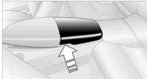
To open, raise the cover at the left or right edge. The compartment contains the cup holder and the lock for the hotel function, refer to page 33.
