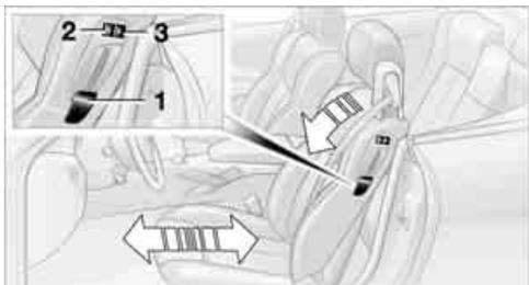
The belt system integrated in the seat makes it easier to get in back.
