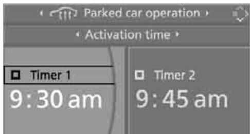
6. Select the time and press the controller. The first time setting is highlighted.
