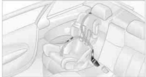
All rear safety belts and the safety belt for the front passenger can be locked against pulling out to secure child restraint systems.
