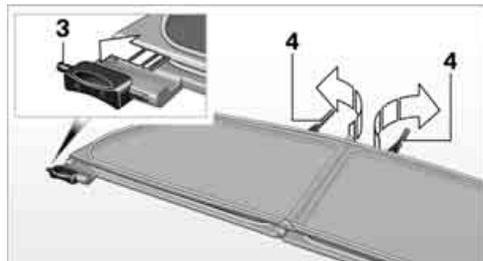
4. Unfold the rear mounts 4.
