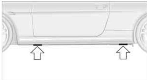
The jacking points for the car jack are located in the positions shown.
