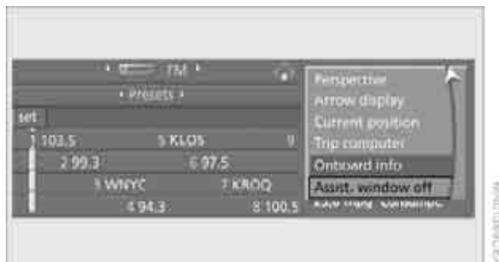
To switch on, change to the assistance window and press the controller.
