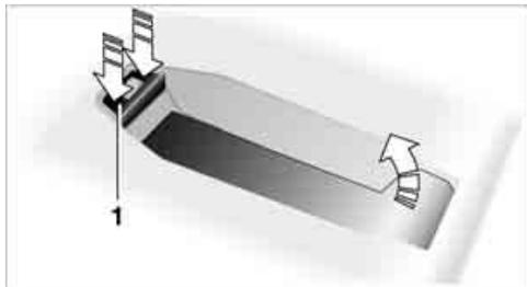
2. Insert the snap-in adapter at the front and press down until it engages.
