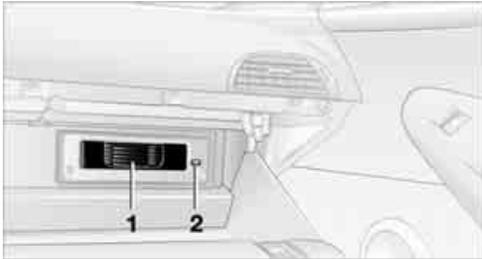
Press button **2** to eject the CD magazine **1**.
