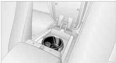
The compartment of the rear center console contains a built-in cup holder and a removable one.
