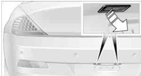
Bulb 5 watts, WY 5 W
