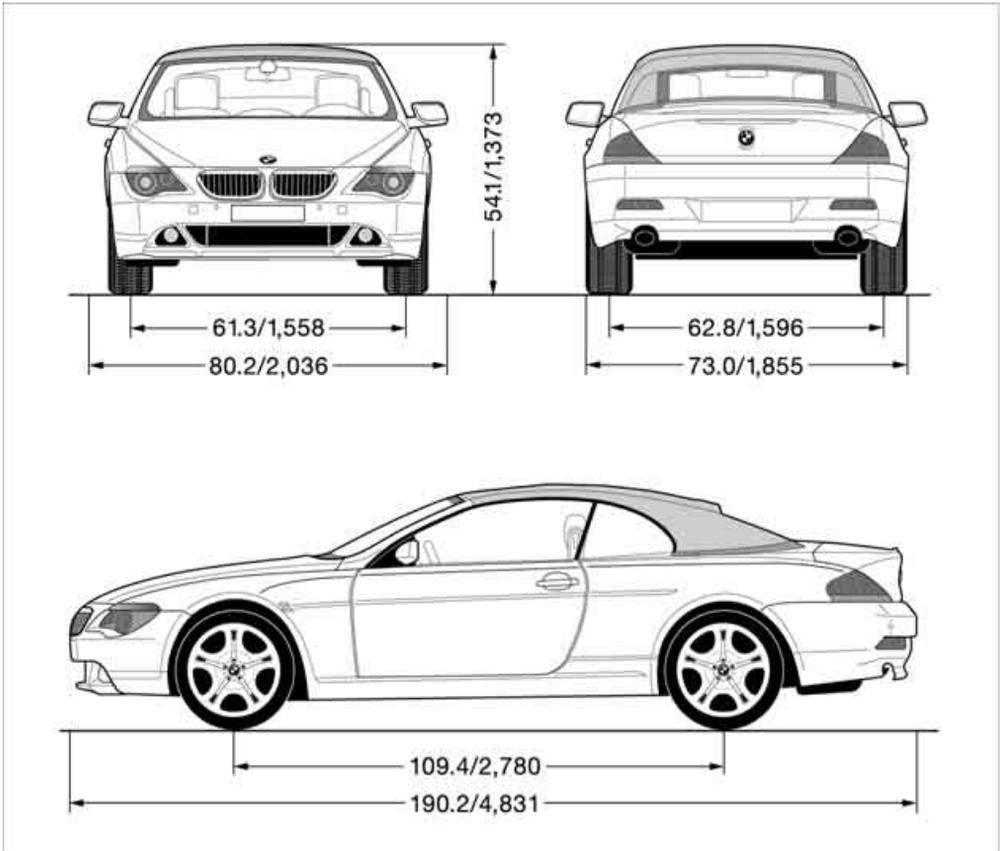
All dimensions given in inches/mm. Smallest turning circle diam.: 37.4 ft/11.4 m
