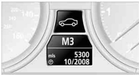
The remaining driving distance and the date for the next maintenance are displayed briefly with the ignition switched on.
