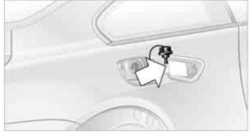
Place the fuel filler cap in the bracket attached to the fuel filler door.
