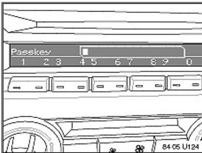
15. Using the soft-keys of the radio enter a user selectable passkey from 4 to 16 digits.
