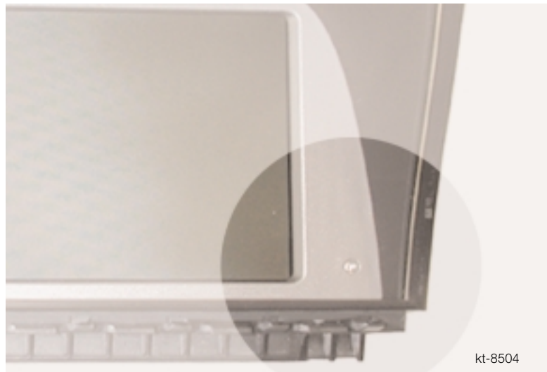
Control Display photo-cell location
