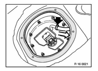
Disconnect the fuel pipe with special tool 13 3 010 and open the hose clamp. Petrol-driven vehicles - inlet line Diesel-driven vehicles - return line
