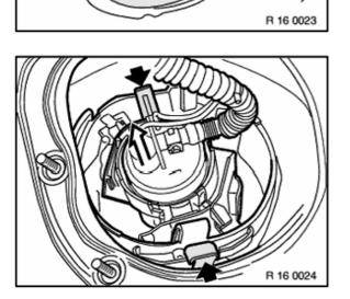
Compress retaining hook on fuel pump (black housing). Remove fuel pump from fuel baffle (white housing).
