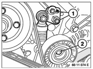
Slacken screws (1) and relieve tension on belt drive.
