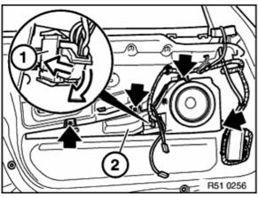
Press down connector fastener, slide lever downwards and remove connector (1) (loudspeaker).
