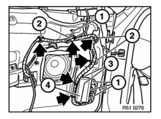
Unlock connector (1) and remove. Unfasten screws (3) and remove control unit (4).
