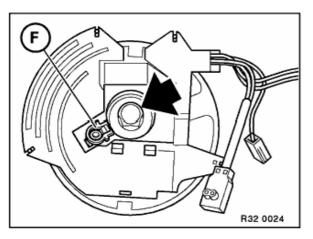
Move steering wheel to straight-ahead drive setting (markings flush on steering gear and steering spindle).
