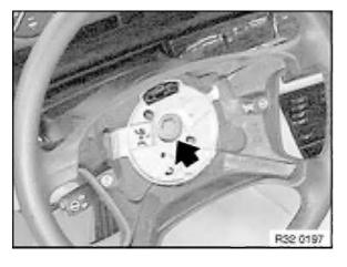
Move steering wheel/wheels to straight-ahead position. Release screw and remove steering wheel.
