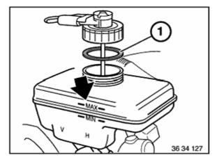
Fill expansion tank up to "MAX" mark with new brake fluid, refer to BMW Service Operating Fluids.
