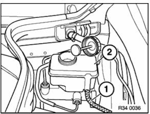
Pull off supply hose on clutch hydraulics (1).
