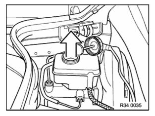
Suck the brake fluid out of the expansion tank. Use a suction bottle used exclusively for drawing off brake fluid.
