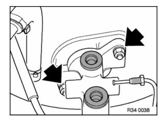
Loosen the nuts and pull the master brake cylinder out of the brake unit.
