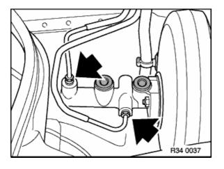
Loosen the screw connections of the brake lines.
