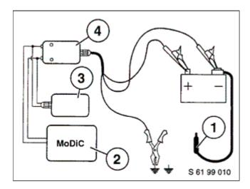
Connect (3) MoDiC adapter 61 2 310 in parallel to (4) adapter for closed-circuit current measurement 61 3 300. Connect measuring lead MFK1 to MoDiC (2) and select **multimeter** measurement function **voltage V** in the mask.
