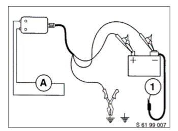
To measure the closed-circuit current, connect the multimeter to the adapter and then unscrew the battery ground lead (1) from the central ground terminal point on the body.
