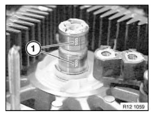
Check contact surfaces of collector rings for wear and recondition if necessary.
