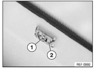
Version with head airbag (ITS): Unscrew bolt (1).
