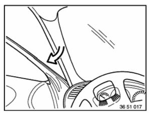
Remove A-pillar finisher by pulling inwards and upwards.
